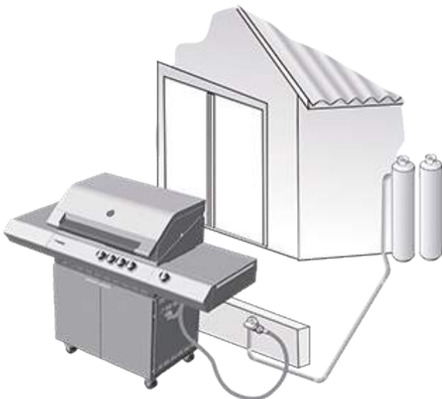
Barbeque connected to twin 45kg LPG cylinders. Copper pipe brings the gas from the tanks to the barbeque area. A flexible hose connects to a bayonet fitting near the barbeque.
