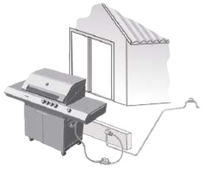
Barbeque connected to the Natural Gas supply. Copper pipe brings the gas from the gas meter to the barbeque area. A flexible hose connects to a bayonet fitting near the barbeque.
